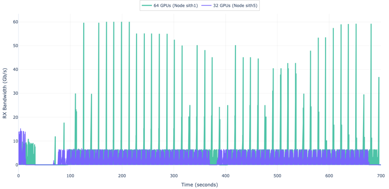
Fig. 2. RX bandwidth utilization during training. The 64-GPU configuration shows periodic bursts up to 60 Gb/s (15% of 400 Gb/s capacity), while 32 GPUs maintains steady 6 Gb/s.
